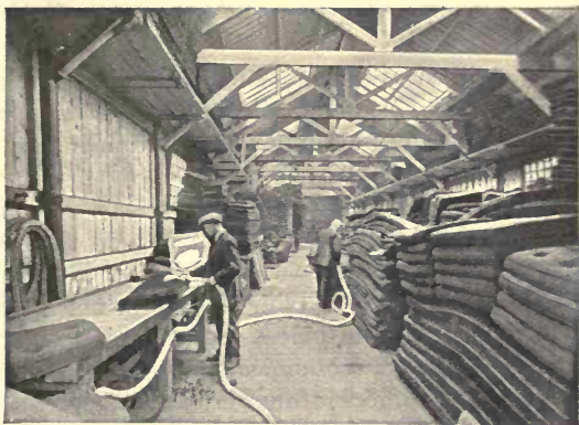
FIG. 31.—SUCTION CLEANING FOR RAILWAY CARRIAGE CUSHIONS.
